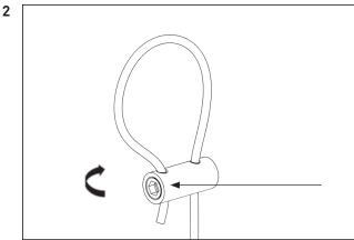
Loosen the screws on both sides to adjust the wire, and cut if needed to find the correct length.
