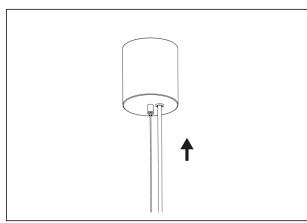
Attach the wire to the hook, and make sure the lamp is in the correct heigh
