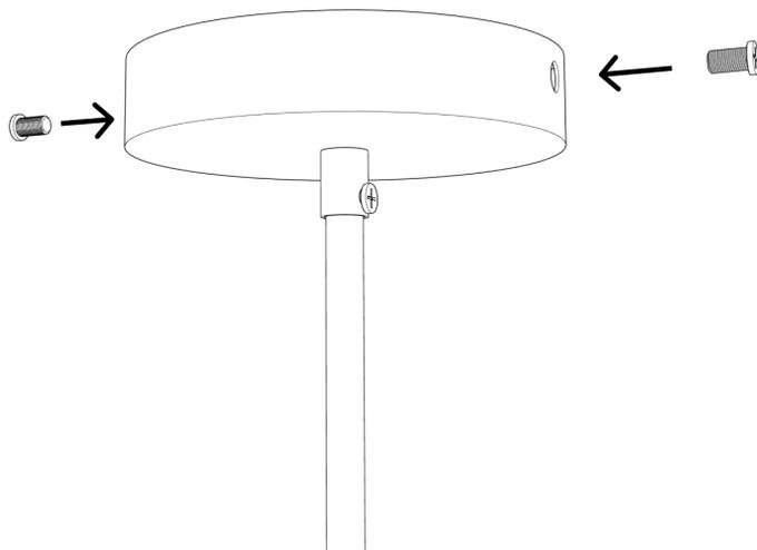
**Step 4** Place the canopy cup onto the metal bracket and secure it in the right position with the including screws.
