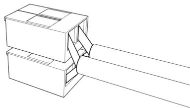
**Step 3** Use the terminal boxes (C) to assemble the wires from the pendant with the wires from the power supply. Place the terminal boxes inside the canopy.
