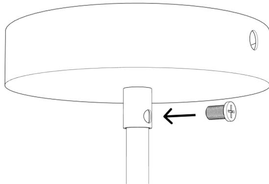
**Step 2** To determine the right suspension height for the lamp, pass the electrical cord through the strain relief of the canopy (B). When you have the desired suspension height of the lamp, tighten the plastic screw of the strain relief.
