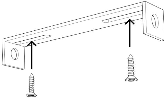
**Step 1** Ensure power supply is turned off and remove any existing lamp fitting. Mount the metal bracket (B) securely in the ceiling with screws and wall plugs, appropriate for the ceiling of installation.
