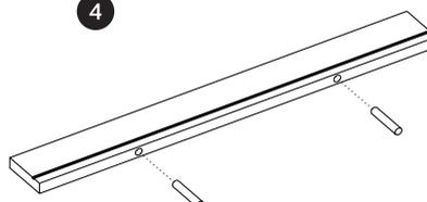
Push the two pins as far into the holes as possible.
