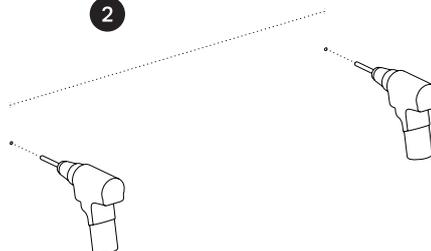
Drill the two holes and insert adequate wall plugs suited for you wall type.
