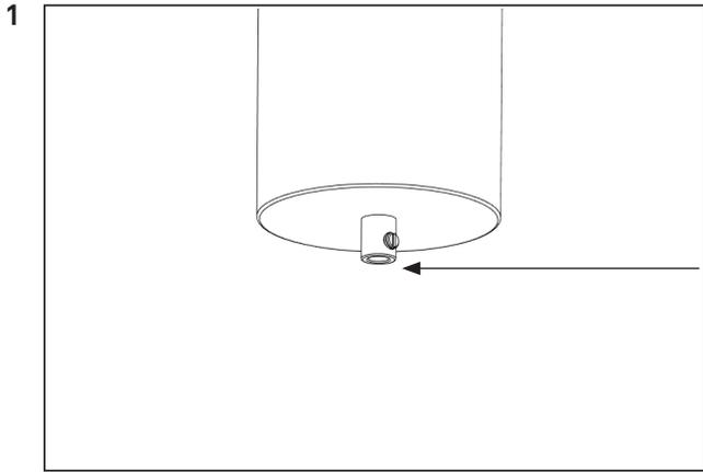
Loosen screw counterclockwise so the cable can pass.
