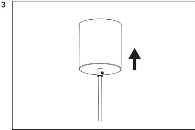
When the lamp is mounted properly to the ceiling, slide the canopy to the ceiling.
