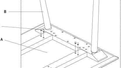
Slot  ${\bf B}$  into  ${\bf A}$  and fix into position using  ${\bf E}$  as shown above.
