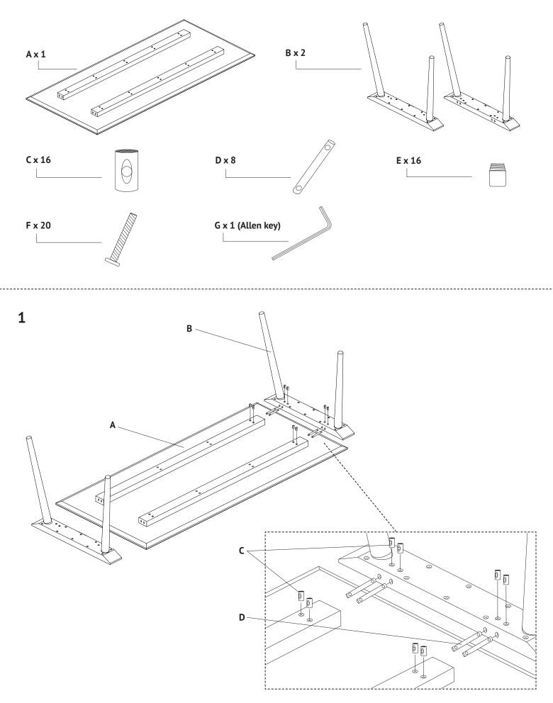
First insert  ${\bf C}$  into the eight holes shown above. Then insert  ${\bf D}$  into corresponding holes. Repeat on oposite side of the table.
