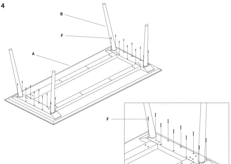
Securely tighten the table top and legs together using parts  ${\bf F}$  and  ${\bf G}$  (Allen key). Repeat on oposite side.
