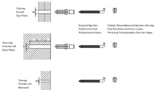
Template for drilling for mounting screws.
