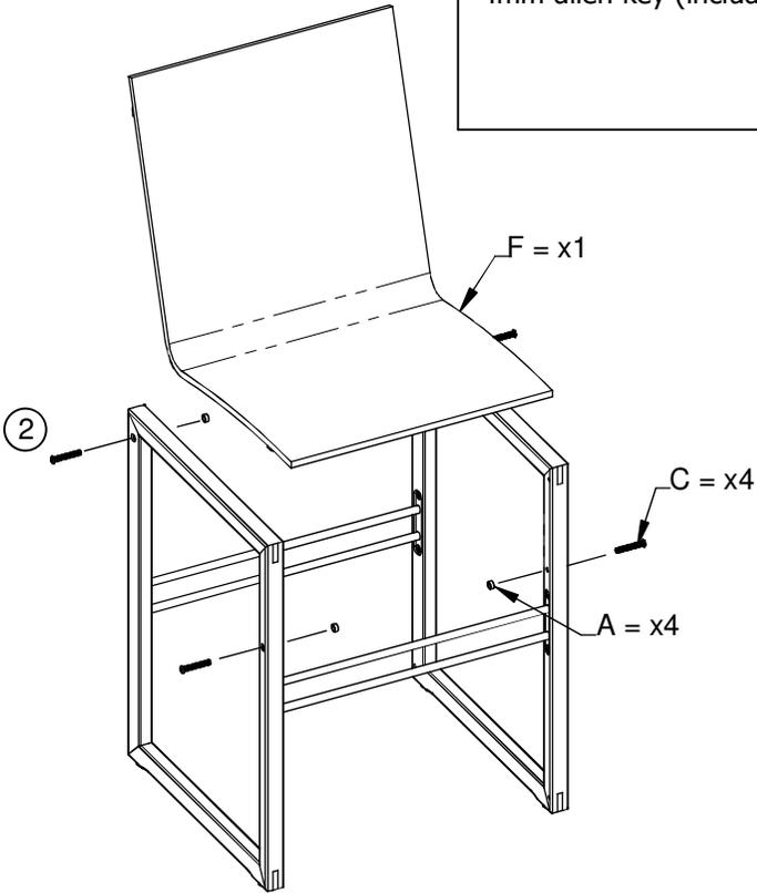
2a. Line the seat/back assembly up with the 4 upper holes in the teak frames and secure them loosely in place (two turns only) with the custom bolt M8x50mm - Note that there must be Ø12x7mm spacers between the teak frames and the seat assembly
