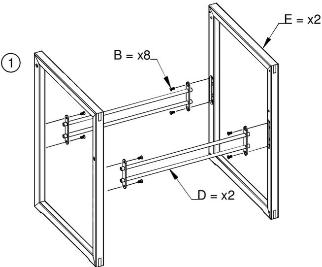
1. Secure the four stainless steel tubes in place using the supplied allen key and 8pcs M6x16mm bolts - Do not fully tighten the bolts, instead secure them loosely in place with two turns only
