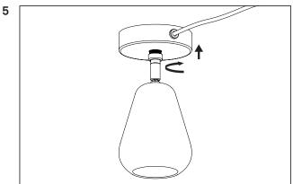
Slide the cover plate against the mounting surface. Secure it with the finger screw.
