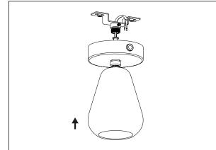
Reattach the lamp by inserting it into the bracket and tighten the set screw.
