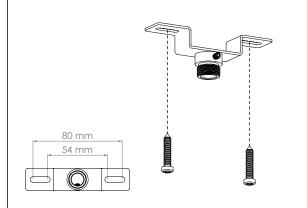
Attach the mounting bracket to the wall or ceiling with screws. (Not included)
