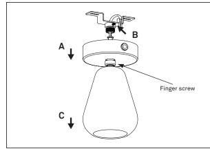
A: Disassemble the lamp from bracket by unscrewing the finger nut and slide the canopy cover towards the shade.
