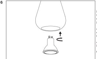
Place a GU10 light bulb in the socket by inserting it and twisting clockwise. The bulb is NOT included.
