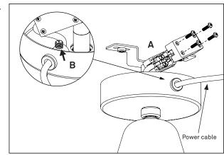
A: Connect the lamp cable to the cable terminal inside the connector box.
